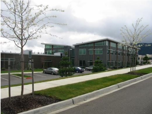
Shown Above: A massing offset in height and façade depth helps break down the apparent mass of this commercial/industrial building.
